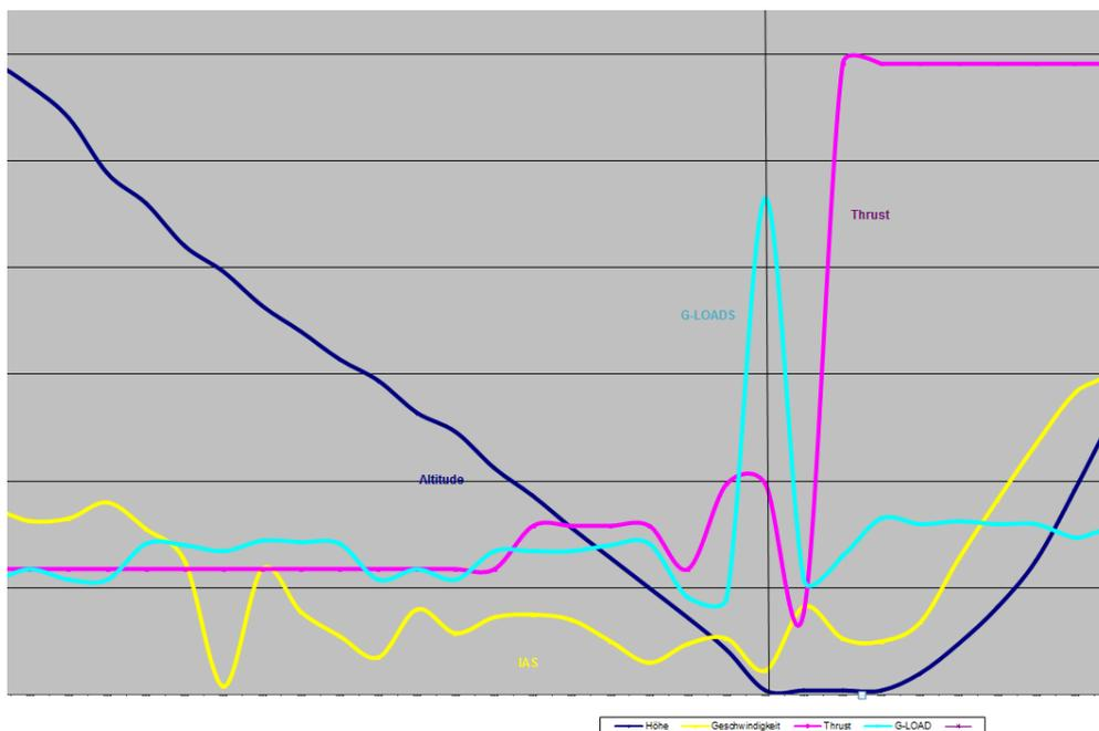
**Figure 1.** Curves for the altitude, IAS, thrust and G-load parameters during hard landing
