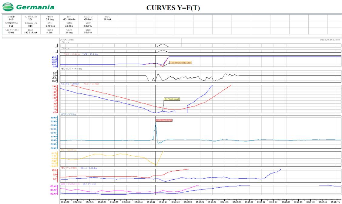
**Figure 2.** Graphs for the main DFDR parameters during the approach and landing
