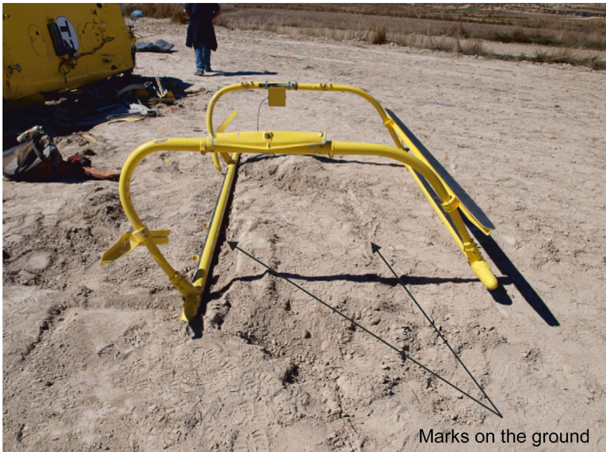
Figure 10. Bent landing gear and marks on the ground
