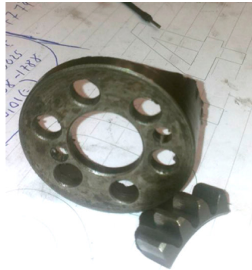
Figure 4. Broken gear installed in the engine
