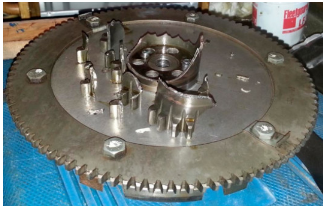
Figure 3. Flywheel and damaged cone gear
