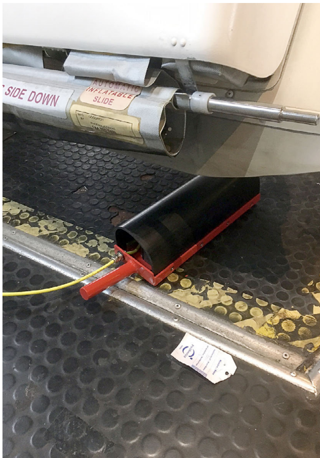
Figure 2. Positioning of the safety shoe between the door and the finger floor
