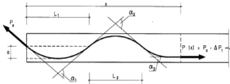
If  $a \leq 0.045 L_1$  then  $\alpha_1$  may be taken as  $\alpha_1 = \frac{8a}{L_1}$ ; being the error less than 5%
