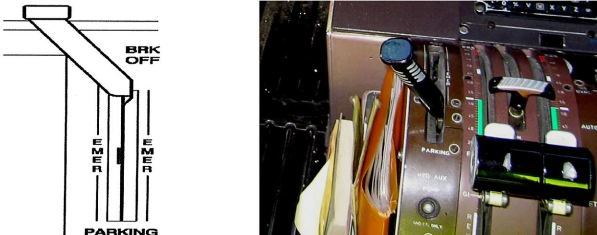
Figure 5. Photograph of the parking brake lever (right) and diagram showing its positions (left)
