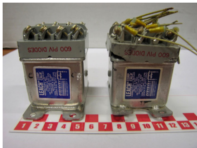
Figure 8. Comparison between the recovered relay and a new one of the same model
