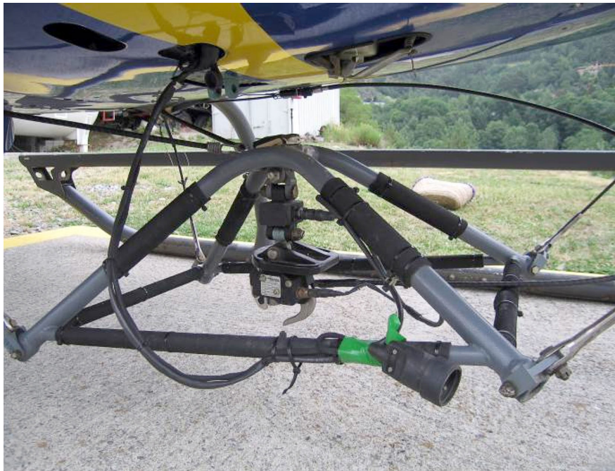
Figure 3. Structure of the CARGO SWING unit similar to the one on the accident helicopter
