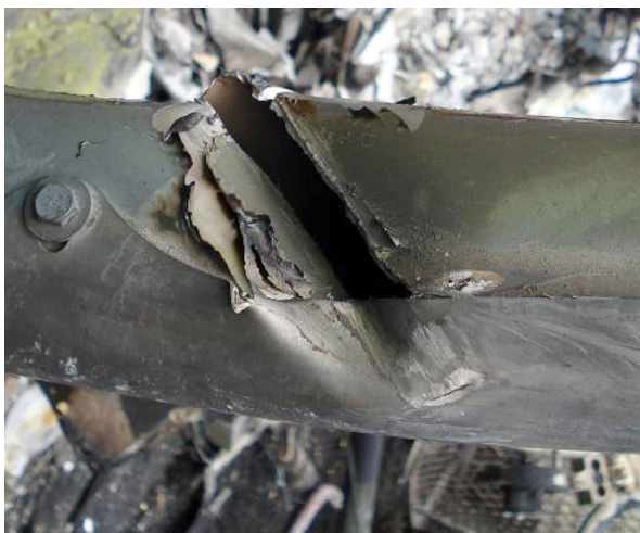
Figure 8. Damage to the right skid
