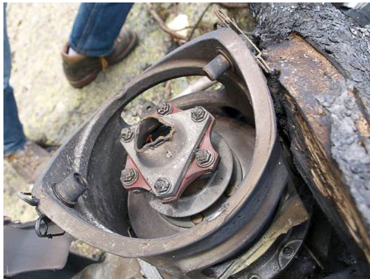
Figure 10. Fracture of the main driveshaft on the BTP side
