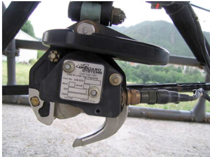
Figure 16. Hook similar to the one in the accident, in the open position
