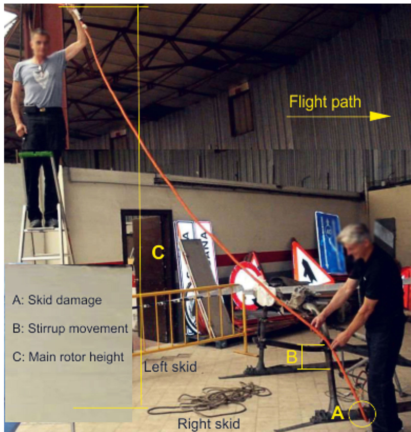
Figure 15. Reconstruction of the position of the sling in the rotor blades
