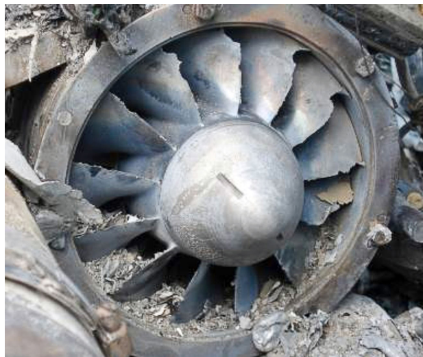
Figure 11. Damage to the blades
