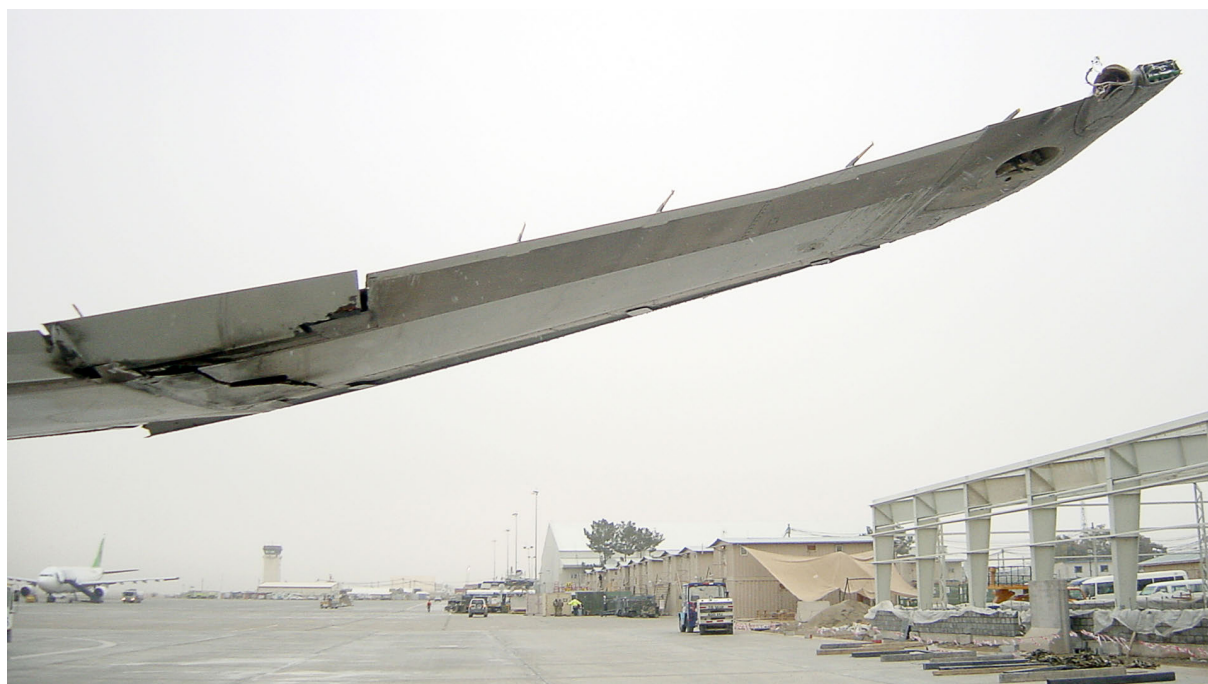
Figure 1. Damaged right wing seen from behind
